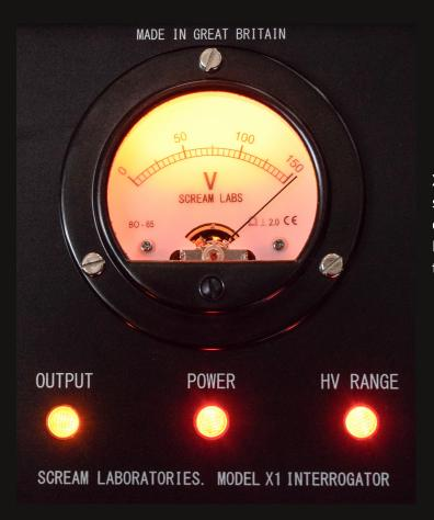
X1 units are fitted with a high quality, retro style, phenolic case meter that is back-lit for easy visibility in low light environments.
