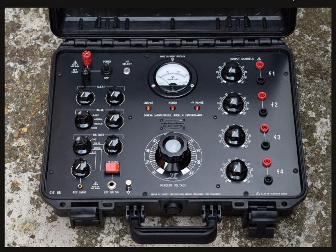
The MAX is fitted with a 58mm diameter central voltage knob with highly visible retro style dial.
